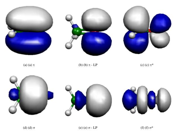
Fig. 7.63: Six NBOs of the  $H_2CO$  molecule. Shown are the occupied bonding  $\pi$  and  $\sigma$  orbitals (left) for C and O, the two oxygen lone pairs (middle) and the two  $\pi^*$  and  $\sigma^*$  antibonding orbitals (right).
