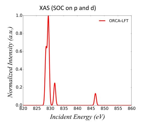
Fig. 7.71: orca\_lft simulated  $Ni^{2+}$  L-edge XAS spectrum
