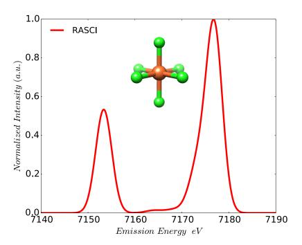
Fig. 7.42: Calculated RASCI  $K_{\beta}$  XES spectrum of  $[Fe(Cl)_{6}]^{+}$ .
