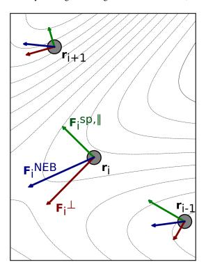
Fig. 7.21: Visualization of the effective force,  $F^{\text{NEB}}$  and its two components:  $F_i^{\perp}$  and  $F_i^{\text{sp},\parallel}$  for three images along an intermediate path in a NEB optimization. The figure is taken from Ref. [3]
