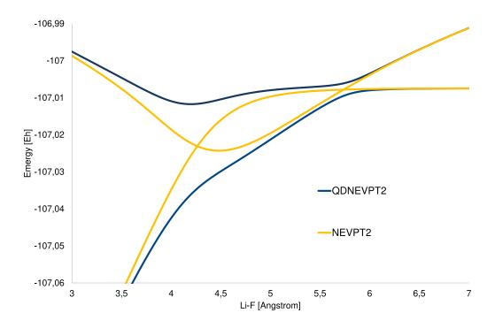
Fig. 7.7: SC-NEVPT2 and QD-SC-NEVPT2 Li-F dissociation curves of the ground and first excited states for a CAS(2,2) reference
