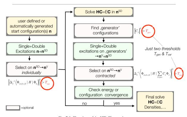
Fig. 7.8: Flowchart of the ICE-CI procedure.
