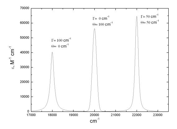
Fig. 7.43: Absorption spectrum generated after orca\_asa run on file example001.inp. Three bands have different lineshape pararameters. Note that although all transitions are characterized by the same transition electric dipole moment their intensities are scaled proportionally to the transition energies.
