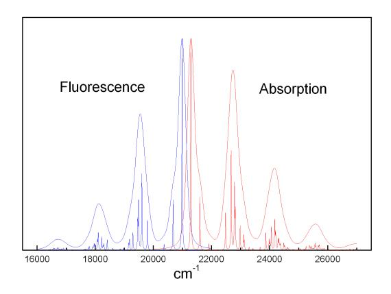
Fig. 7.44: Absorption and fluorescence spectra generated after orca\_asa run on the file example002.inp. If the homogeneous broadening is set to be  $\Gamma=10\,\mathrm{cm}^{-1}$  one can resolve underlying vibrational structure and identify various fundamental and combination transitions.
