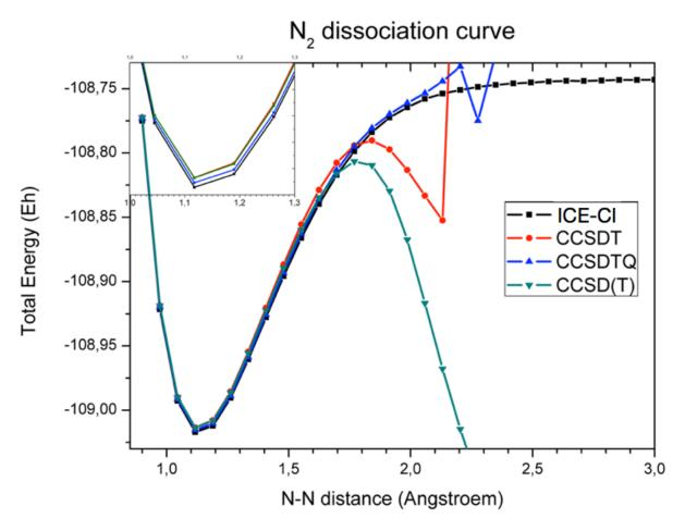
Fig. 7.14: Potential energy surface of the  $N_2$  molecule in the SV basis. For comparison higher level coupled-cluster results are also shown.
