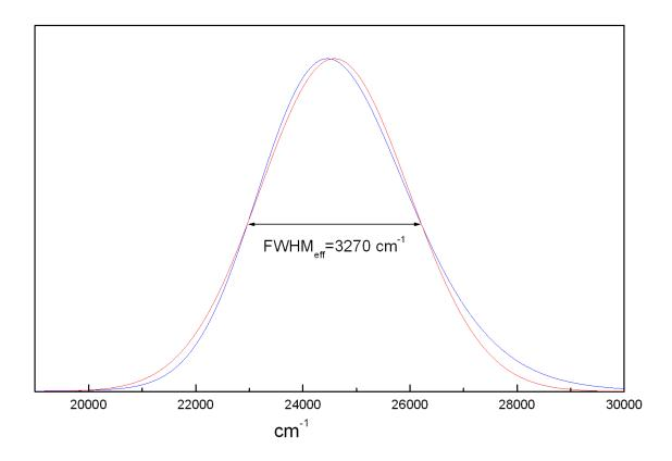
Fig. 7.47: Absorption spectrum (blue) for  $T=300~{\rm K}$  generated after orca\_asa run on the file example004.inp. Red line represents the Gauss-fit of the calculated spectrum.
