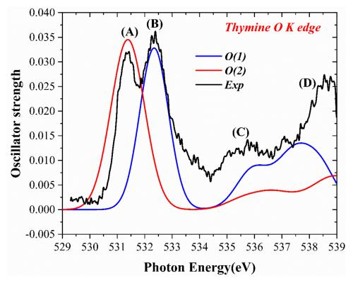
Fig. 7.39: Comparison of theoretical and experimental X-ray absorption spectra of oxygen K-edge in thymine. The simulated spectrum is shifted by -3.7 eV to align with the experimental spectrum.
