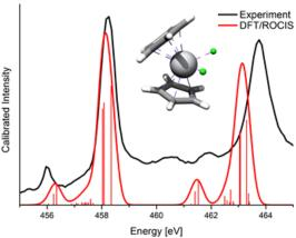
Fig. 7.32: Comparison of the experimentally observed (black) and calculated (red) Ti L-edge of  $[Cp_2TiCl_2]$ . The red bars highlight the contribution of the individual states to the total spectrum. The pure ROCIS method (left) predicts a wrong  $L_3$ - $L_2$  intensity ratio and strongly overestimates the splitting of the satellite features to the main bands. Better results are obtained with the DFT/ROCIS method (right).
